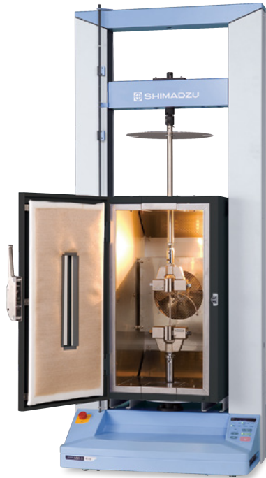
AGS-10kNXD + Screw Type Flat Grips + TCE series Compact Thermostatic Chamber
