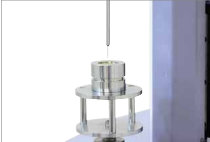
⑭ Boil-in-bag piercing stand ⑮ Upper jig ⑯ Lower jig
