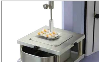
④ Tablet press-dispense jig set ⑤ Jig platform ② Upper jig
