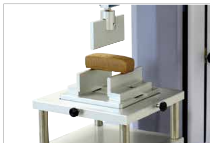
⑳ Three-point bending test jig (R2.5mm) ⑩ Jig platform
