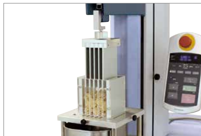
⑯ Kramer shear cell, 5-blade type ⑩ Jig platform
