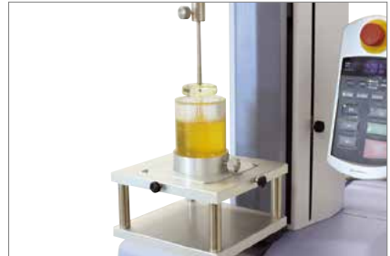
⑧ Overflow test jig set ④ Jig platform ⑤ Upper jig
