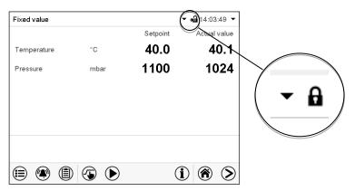
In the locked view the controller provides all display functions. No setting functions are available.
