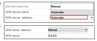
After completing the settings, press the **Confirm** icon to take over the entries and exit the menu, **or** press the **Close** icon to exit the menu without taking over the entries.
