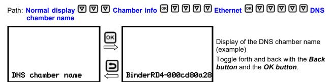
With the **Back button** you can go back to the "Ethernet" submenu and, repeatedly pressing it, to Normal display.
