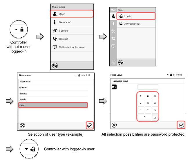
After completing the settings, press the *Confirm* icon to take over the entries and exit the menu, **or** press the *Close* icon to exit the menu without taking over the entries.
