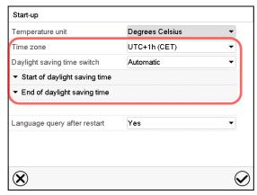
Select the time zone and configure the daylight-saving time switch.
