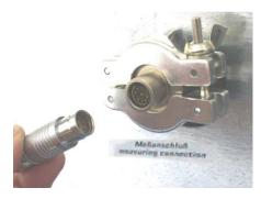
Figure 25: Measuring connection (12) with measuring access port
