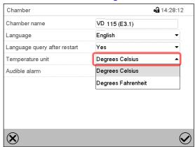
Select the desired temperature unit and press the *Confirm* icon.
