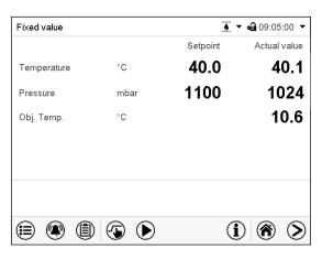
Normal display with object temperature display (sample values)
