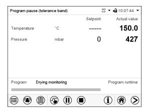
Normal display. Information on the bottom of the screen indicates the currently running program and the time already passed. The grey bar shows how much time of the whole time is elapsed.
