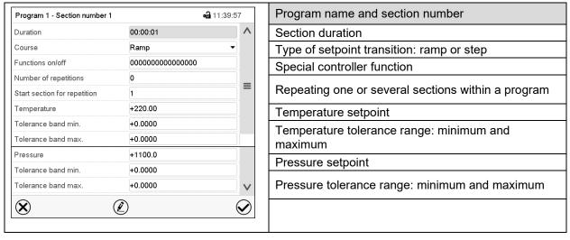
The setting and control ranges for the individual parameters are the same as for "Fixed value" operating mode.
