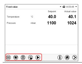
Use the **navigation icons** in the screen footer in Normal display to access the desired controller functions.
