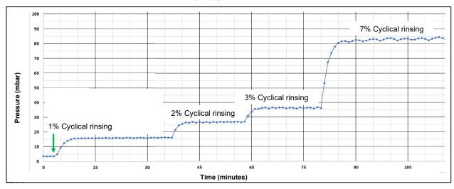
Figure 22: Pressure curve depending on the setting values for cyclic rinsing, sample representation beginning at the final vacuum of 4mbar VD 56 with VAP 2
