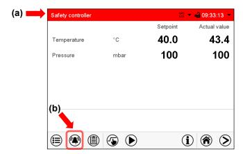
Normal display in state of alarm (example).
