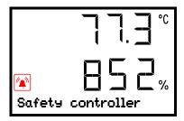
Alarm indication (example: safety controller alarm) (sample values)
