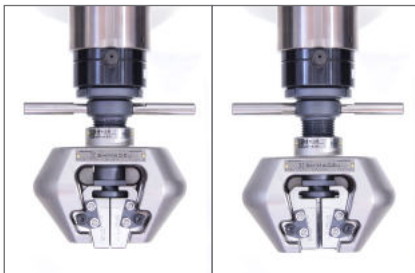
The grip faces stay in the same vertical position
