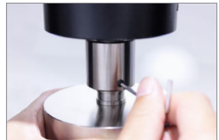
Connect the joint and plate, and fix by screw
