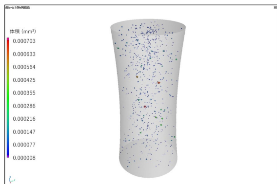
Fig. 4 Void distribution on specimen 1
