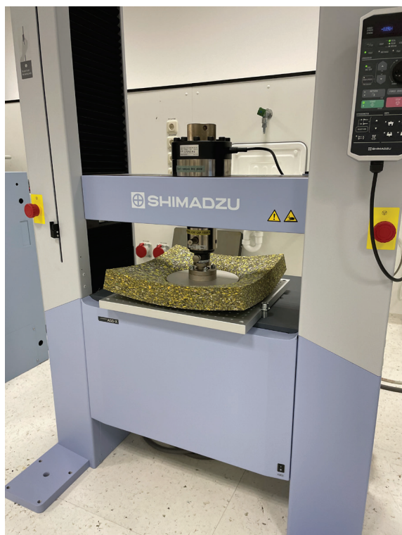
Fig 3 deformation of sample after indentation loading
