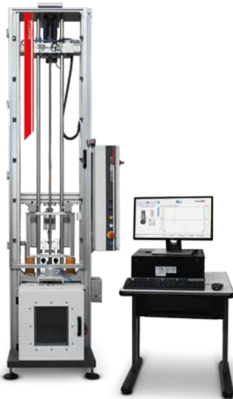
Drop Weight Tower with climatic chamber DW625
