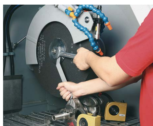
Easy Exchange of Cut Off Wheel
