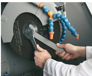
Easy Exchange of Cut Off Wheel
