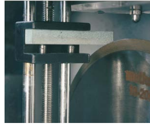
Blade dresser available for dressing even during cutting
