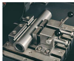
Stainless steel clamping devices and T-Slotted table
