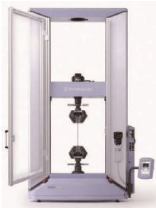
Fig. 1 Overview of Universal Testing System
