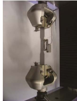
Fig. 2 Specimen and Jigs for Tensile Testing
