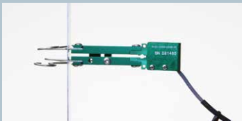
Model 3442 with 6.0 mm gauge length and \pm 5.0 mm/ -1.0 mm ( +83\% / -17\% strain) measuring range
