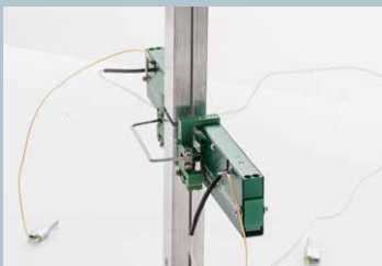
Side view of the Model 4013 lap shear extensometer with zero pins removed
