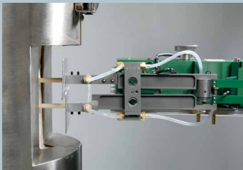
Model 3648 with 1 inch gauge length
