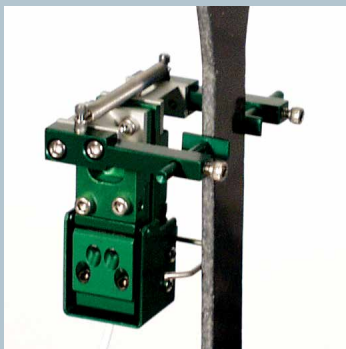
Model 3475-050T-ST with \pm 0.050 inch measuring range
