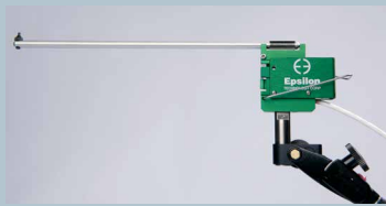
Model 3540 with 25 mm measuring range
