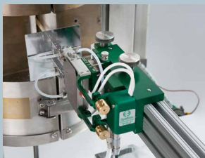
Model 3549 with 25 mm gauge length
