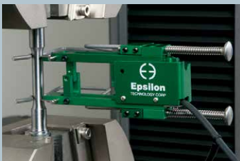
Model 3542 with round metal specimen
