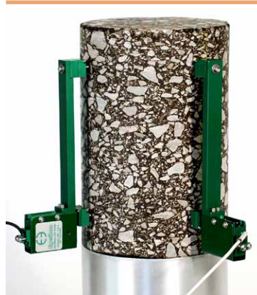
Model 3909-0400 with 4 inch gauge length
