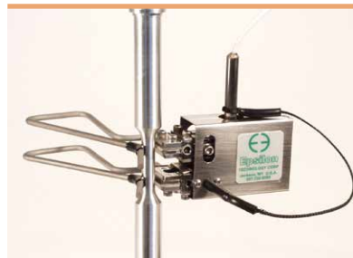
Model 4030 with 0.5 inch gauge length
