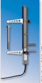
The extensometer system MFD 3 is suitable to determine the strength of pressure (ASTM D-2938) or respecvely the modulus of elasticity (ASTM D-3148) of concrete cylinders under longitudinal compressive stress. The application is carried out with two or three gauge lines.
