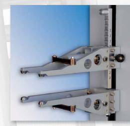
The transverse extensometer MFQ-A (with two measuring locations) - especially when combined with the extensome ters MFL and MFX - is very well suitable for the determination of the r-value of fine sheet metal specimens.
