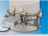
The MFU 4 is suitable for measuring the stac modulus of elasticity and poisson's ratio of concrete in compression in accordance to the standard ASTM C-469.
