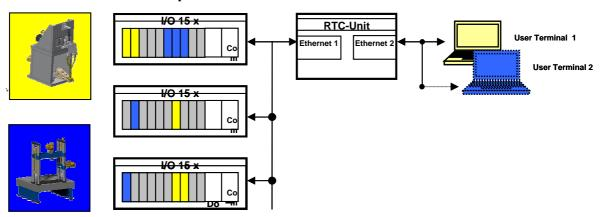
The Multi-Station Multi-User capabilities allows to control several test rig from one or several user terminals. System resources can be assigned freely to any test rig configuration. There is no hard binding from sensor channels to control channels. Each signal can be configured as a control loop feedback signal in depended from the position in the system.
