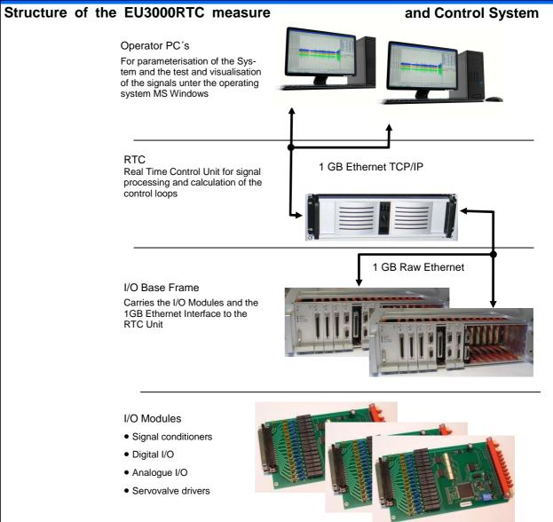
Core element of the EU3000RTC is the RTC Real Time Control Unit. The RTC processes the input and output signals, calculates the PID loop and run the test sequence.
