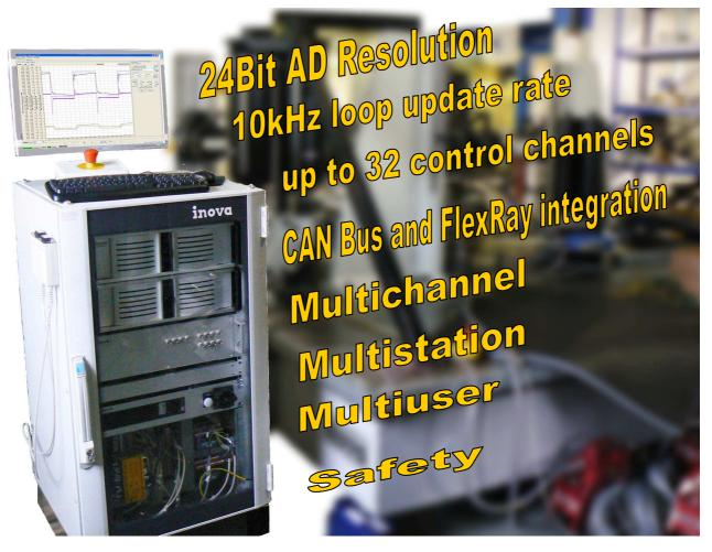
The EU3000D is the newest generation of digital measure and control system. It's fully modular design allows the most flexible set up for all test applications from a simple single channel test rig up to complex cross coupled 32 channel full vehicle simulator.
