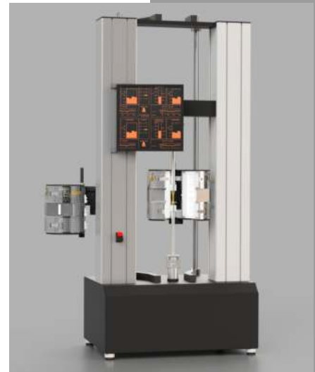
Twin furnaces attached to rear mounted pillars (electromechanical)
