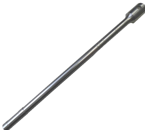
Picture 9: Test piston with piston fixing
