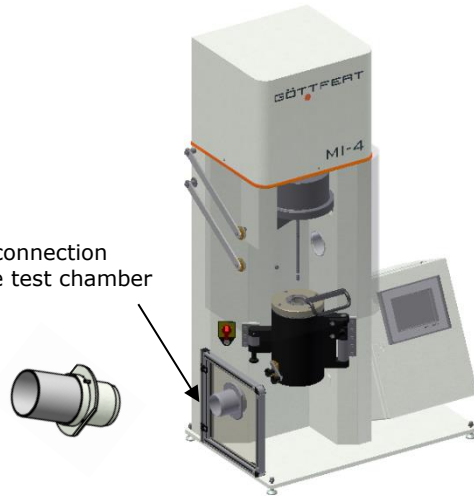
Picture 5: Exhaust connection below
