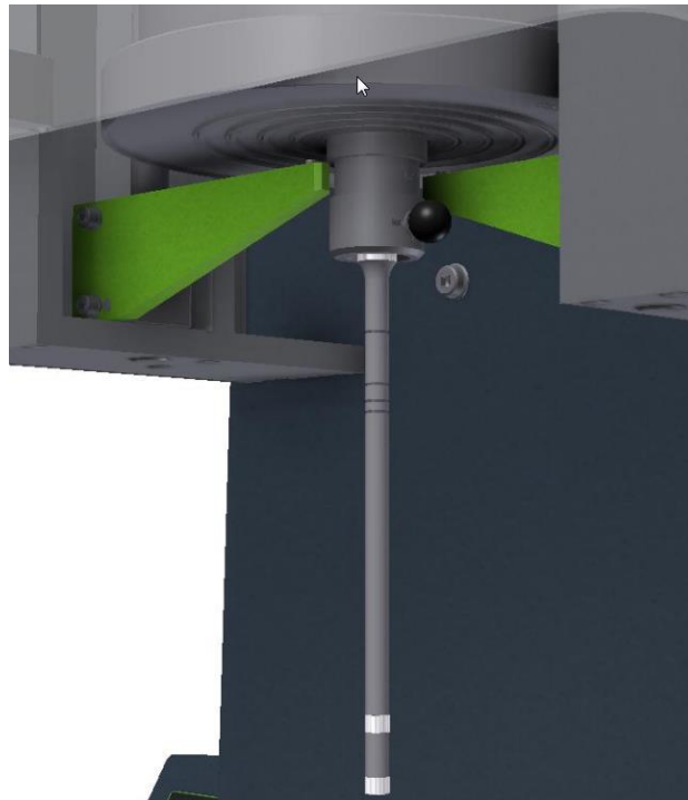
Picture 11: Test piston in optimized test piston fixing
